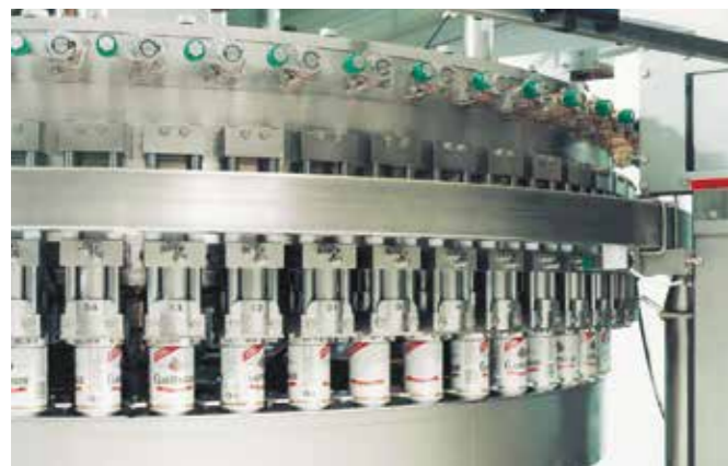
Filling machine, Krones AG, Rosenheim (Germany)
