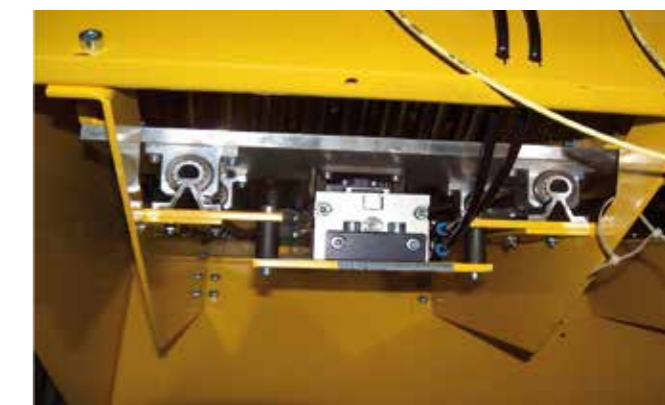
Cost-effective guide for work piece carriage in a machine tool with supported aluminium shaft.
