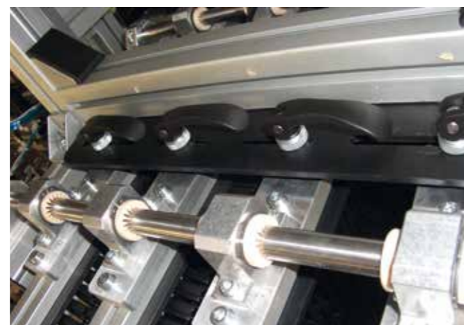
The production line should be adjusted without setup time being required. drylin® linear guides, which enable precise and fast adjustment, were used for this.
