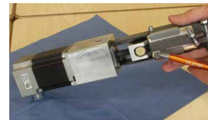
Anti-backlash lead screw nuts in a glue application system of a seam gluing machine (wood industry). These ensure the utmost precision for this clearance-free adjustment drive.
